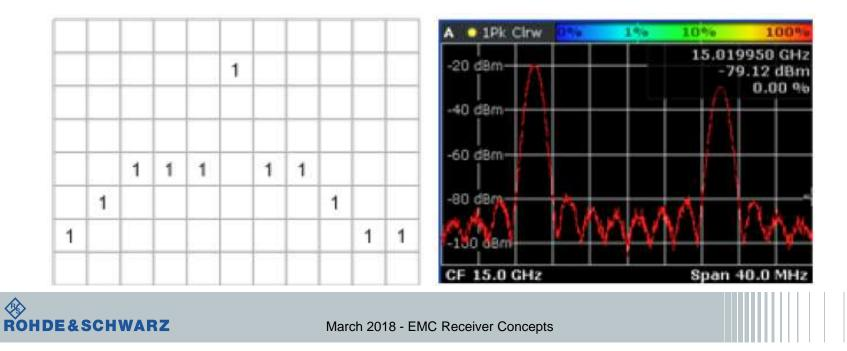
Virtual table and diagram containing the results after one FFT
