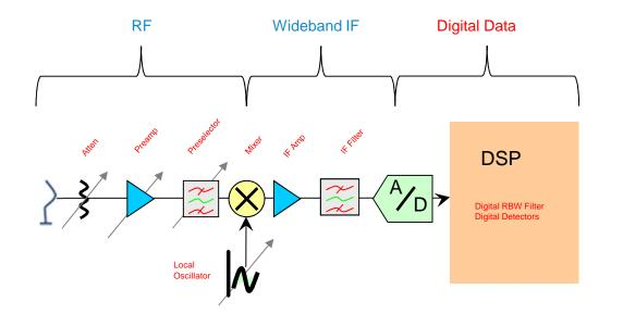
Wideband IF into ADC and digital signal processing provide for a entire new level of feature / functionality including:
