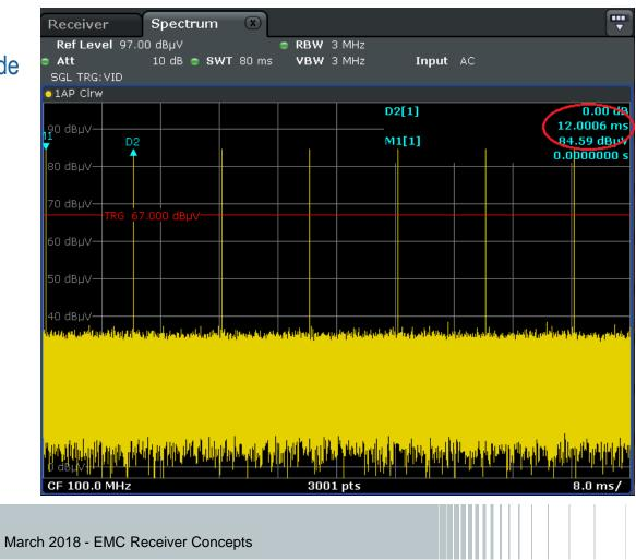
Zero span display in spectrum analyzer measures signal period / pulse repetition rate
