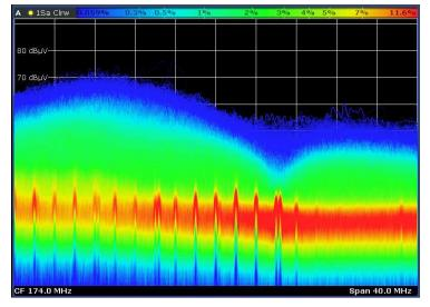
2nd pulsed disturbance signal hidden by the broadband noise, not detectable by conventional spectrum analysis
